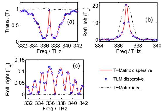
Fig. 2. (a) Transmittance and (b) reflectance for left and (c) right incidence of PTBG as a function of frequency considering a linear medium ( $n_2 = 0$ ) at U condition ( $|\alpha_0| = 1460.24$  cm<sup>-1</sup>) with no gain/loss saturation ( $\mathbb{S} = 1$ ). The results obtained using the T-matrix method for the idealized gain/loss model are included for reference.
