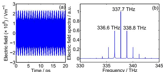
Fig. 5. (a) Time and (b) frequency response of the transmitted electric field of the NPTBG at U operation ( $|\alpha_0| = 1460.24 \text{ cm}^{-1}$ ) with input intensity  $I = 2.6 \times 10^{14} \text{ Wm}^{-2}$  and the incidence from the left side of the grating.
