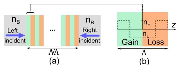
Fig. 1. (a) Schematic of an  $N$ -period PTBG in a background material  $n_B$ , (b) single period of a grating with  $n_H$  and  $n_L$  as the high and low real refractive indices at  $f_B$  in even symmetry and gain (green) and loss (orange) in odd symmetry.
