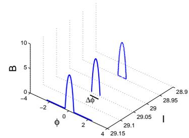
**Figure 1.** Orbits homoclinic to  $\Pi_0 = \{ (x, y, I, \phi) : x = y = 0, 1 < \delta < 3, I > \frac{\Omega_1}{3 - \delta} \}$ . For  $I = I_0$  (the orbit in the middle),  $d\phi/dT = 0$  on  $\Pi_0$ , and the orbit is heteroclinic, connecting fixed points on  $\Pi_0$  that are  $\Delta\phi$  apart. For  $I \leq I_0$ ,  $d\phi/dT \leq 0$  on  $\Pi_0$ . The parameters are  $\delta = 1.49704$ ,  $\Omega = -110$ ,  $\Omega_1 = 27.6085$ .
